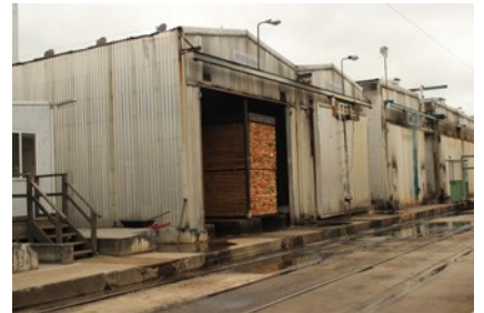
Kiln dried timber is stronger, more stable and less prone to mould or decay.
